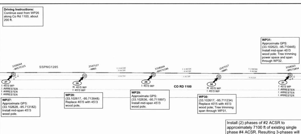
approximately 7100 ft of existing single phase #4 ACSR. Resulting 3-phases will be installed as armless construction. Start at WP1 through to WP38 (S3). NJUNS Ticket # OTH4938764 Remove Type 4H 50 Recloser at WP34 (S8).
